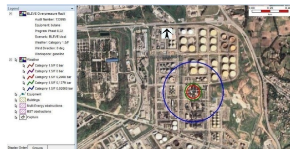
Fig.3 BLEVE Over pressure effects of butane on the refinery
