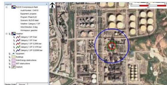
Fig.6 BLEVE Over pressure effects of propane on the refinery
