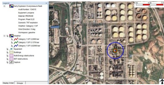
Fig. 7 Early explosion overpressure radiation of propane on the refinery
